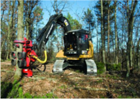
The updated PF-48 fixed processing head, shown here on the Cat® 501HD track harvester, now features a 4-1/2 gallon bar oil tank and other changes designed to increase uptime.
