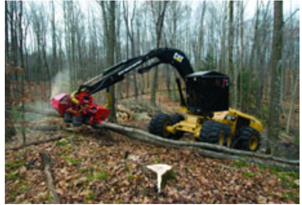
The PF-48, a fixed processing head popular with Lake States loggers, has recently been updated to increase service life and productivity. The robust, simple-to-operate head is shown here mounted on the Cat® 550 rubber tire harvester.
